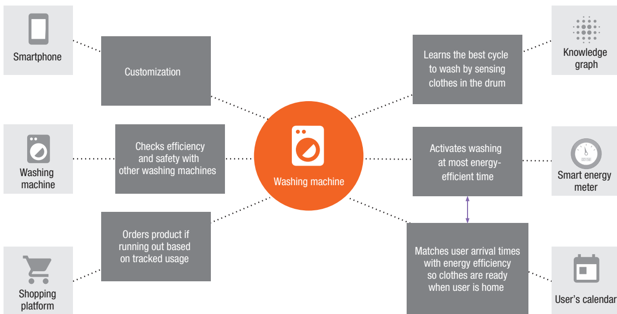
Figure 5. The various features and benefits enabled by connectivity and access to an online ecosystem.
